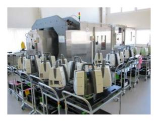
**Figure 13:** A collection of P40 scanners waiting for their turn on the ATEC Calibration Rig. To the human eye, they are perfectly identical, but the human eye is not designed to discern microns. To the Antipodal Telescope Environmental Chamber (ATEC), they are all as uniquely different as human fingerprints.
