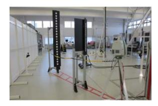
**Figure 19:** A view of the camera calibration stand. Two sets of targets are placed in front of the scanner and are both imaged and scanned.
