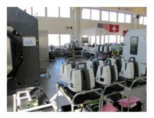
**Figure 10:** A set of P40 laser scanners awaiting calibration on the manufacturing floor in Widnau, Switzerland.
