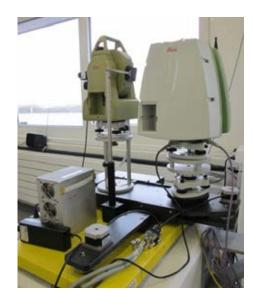
**Figure 18:** Tilt calibration station for the Leica ScanStation C10. The tilt sensor as it is mounted in the scanner is also observed over temperature.
