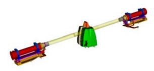
**Figure 16:** Antipodal placement of the ATEC telescopes allows the telescopes to observe their relative placement, when the scanner is removed. This is a patented twist on the idea of auto-collimation techniques that critically allows for arc second level observation and calibration of laser scanners.
