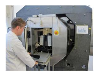
**Figure 14:** A Leica ScanStation P40 being loaded into the ATEC Rig.
