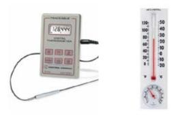
**Figure 6:** The traceable thermometre on the left is far more expensive than the Acurite® thermometer on the right, who uncertainty is not explicitly given.
