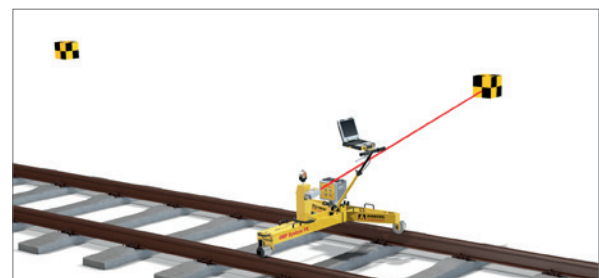
Single control point mode with Amberg IMS 3000 or IMS 1000
